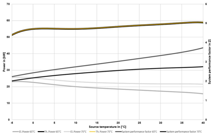
**Figure 2:** Characteristic system curves of the high-temperature heat pump (own representation)
