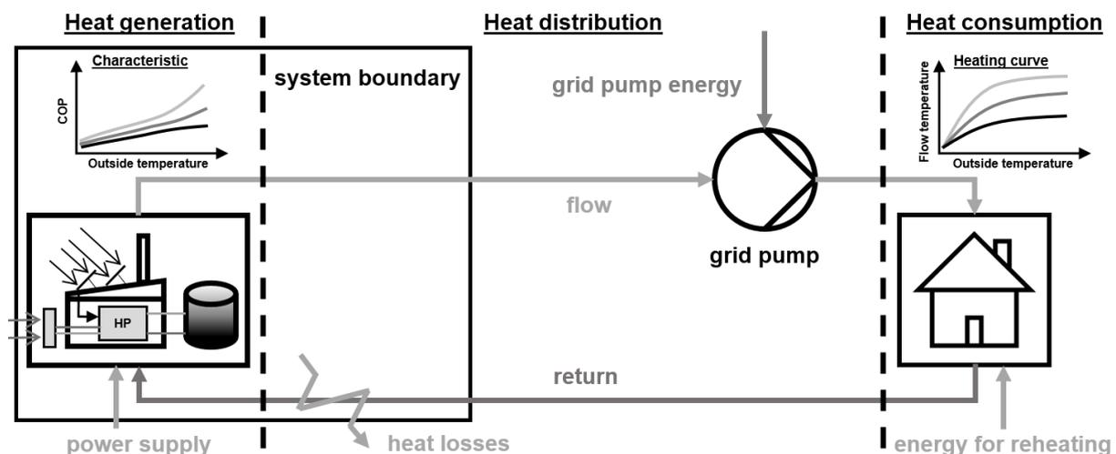
**Figure 1:** System boundary of the heat network calculations for evaluating the economic efficiency of a high-temperature heat pump (own representation)
