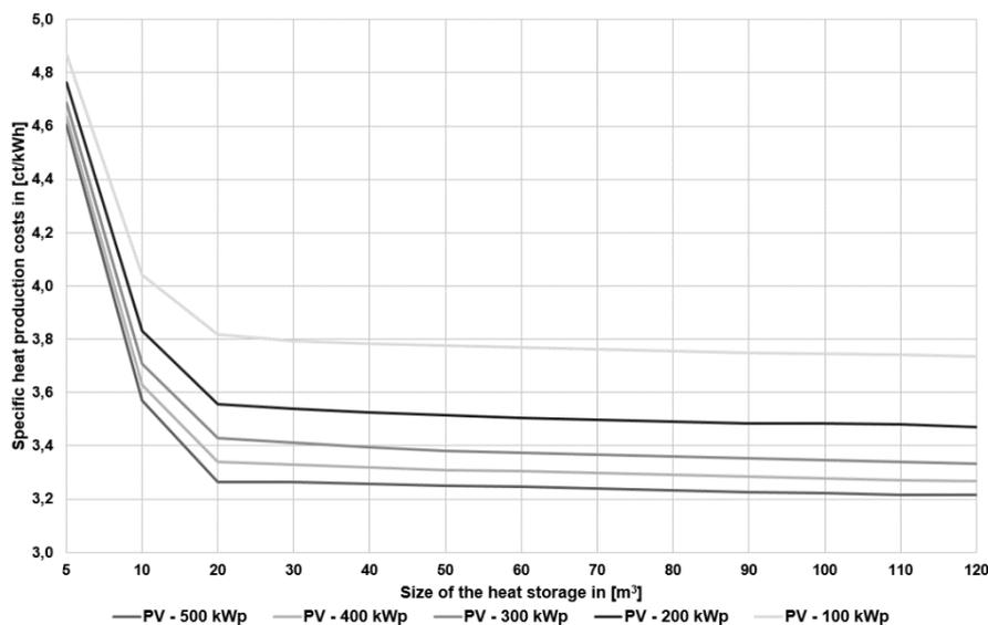
Figure 5: Comparison of the specific heat production costs for the selection of the storage size (own representation)
