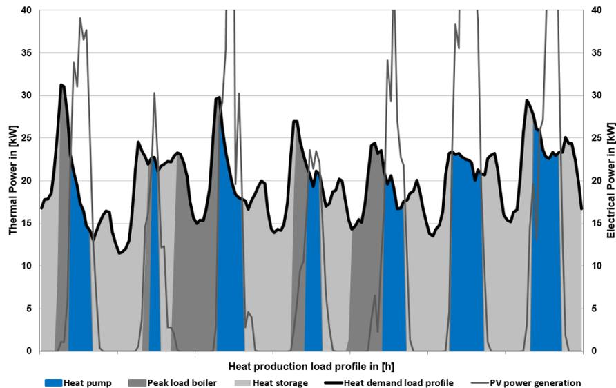
**Figure 9:** Composition of the heat grid feed-in load profile based on a week in April (own representation)
