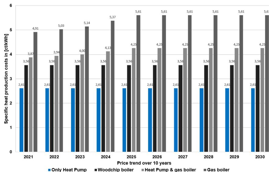
**Figure 11:** Comparison of the specific heat production costs of different forms of heat generation (own representation)
