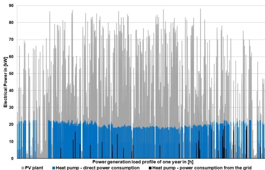
**Figure 8:** PV generation load curve and electricity consumption of the high-temperature heat pump over the course of the year (own representation)
