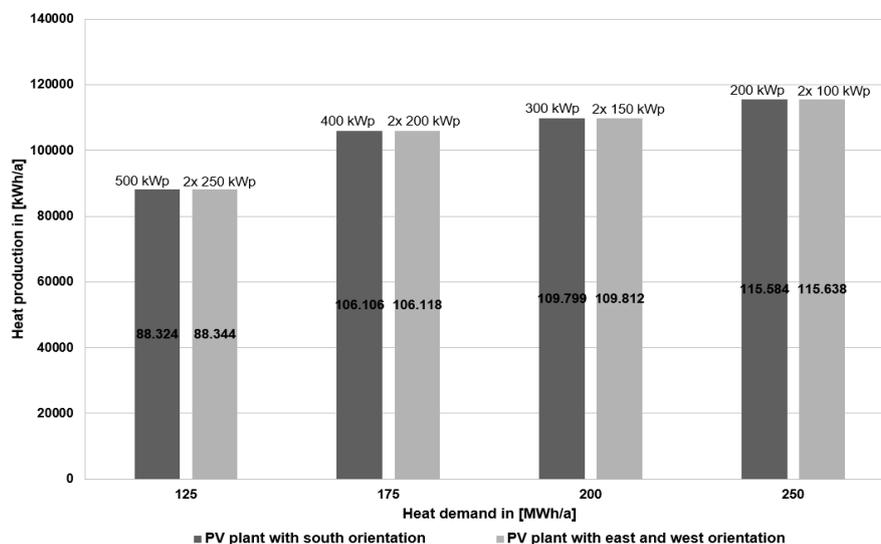
**Figure 3:** Comparison of heat generation amounts based on the availability of electricity from PV systems with south or east-west orientation (own representation)
