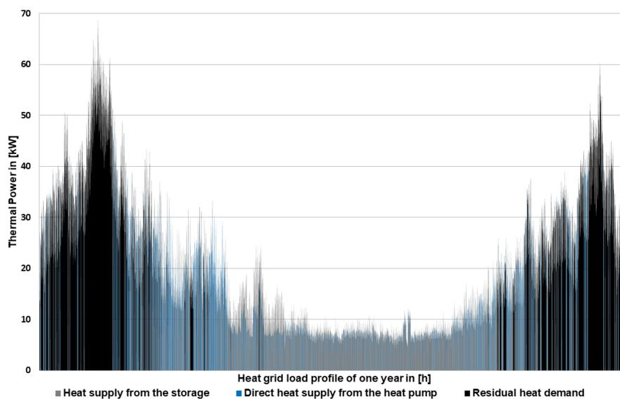
**Figure 7:** Heat supply by the high-temperature heat pump over the course of the year (own representation)
