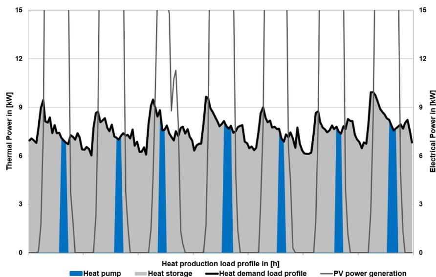
**Figure 10:** Composition of the heat grid feed-in load profile based on a week in July (own representation)
