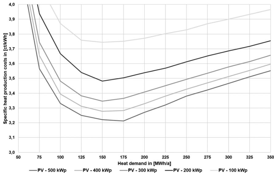
Figure 4: Comparison of the specific heat production costs for the selection of the load profile size (own representation)
