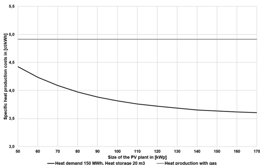
**Figure 6:** Comparison of the specific heat production costs for the selection of the PV system size (own representation)
